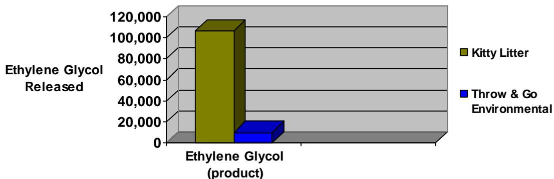
This graph displays results from a TCLP showing how much Ethylene Glycol (anti-freeze) is released from each product in a 20 year landfill simulation.
